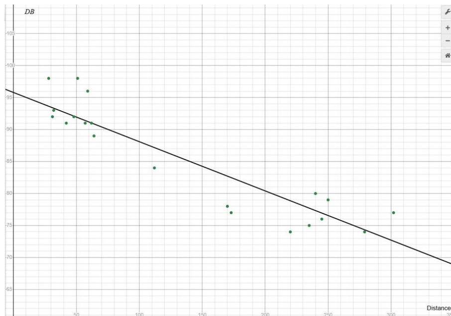
Figure 1 Graph showing DB and distance for all level passes with linear regression
