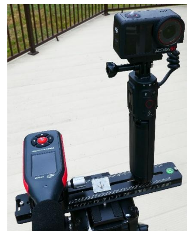
Figure 2 Camera and sound meter on cross bar on tripod
